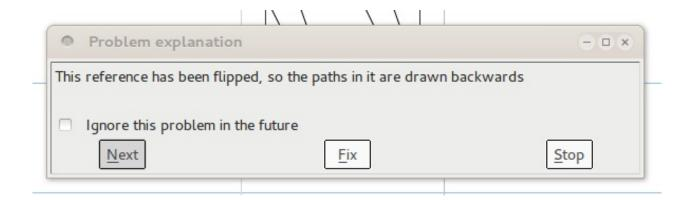
For some problems, there is no automatic fix, but seeing the issue on-screen will help you fix it immediately. For example, a self-intersecting curve has a specific place where the path crosses over itself—it may have been too small for you to notice at a glance, but zooming in will allow you to reshape the path and eliminate the problem.
