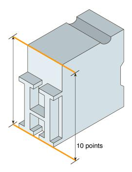
In digital type, the em is a digitally-defined amount of space. In an OpenType font, the UPM – or em size is usually set at 1000 units. In TrueType fonts, the UPM is by convention a power of two, generally set to 1024 or 2048.
