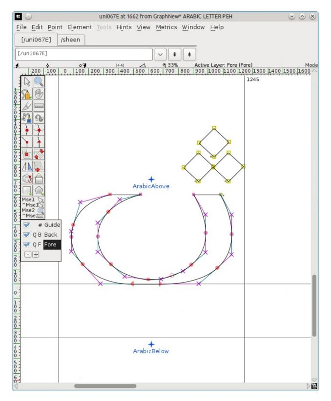
Invert the dots: select the flip tool (two triangles with a red dashed line between them) from the toolbox. (Alternatively, right-click in the middle of the dots, and select **Flip the selection** from the popup.) Click on one of the dot nodes and drag the mouse slightly left or right.
