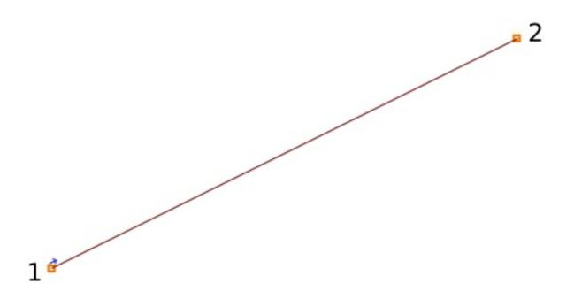
A *Spline* consists of 4 points: 2 end points of the spline and 2 'handles', which describe the slope of the spline at those end points.
