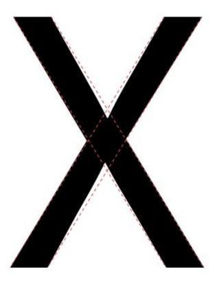
As you can see in this X with dotted line on top of it, the X that appears visually aligned involves an offset.
