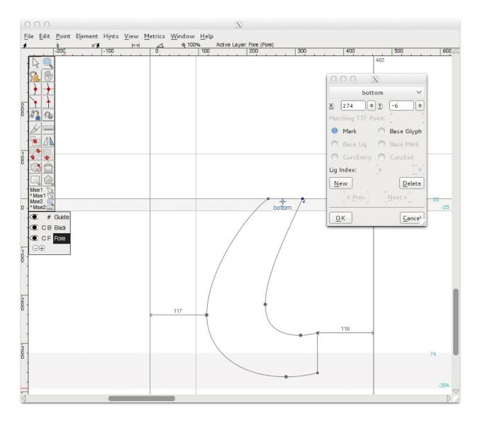
Then, when the 'a ogonek' character is built (using the 'Build Accented Charcter' function) the 'bottom' mark anchor point will be placed at the same location as the 'bottom' base anchor point, ensuring that the referenced ogonek glyph is placed correctly at the foot of the stem of the referenced 'a' glyph (see below). This exact and automatic placement would not have been possible without using anchor points to position the base and mark glyphs.
