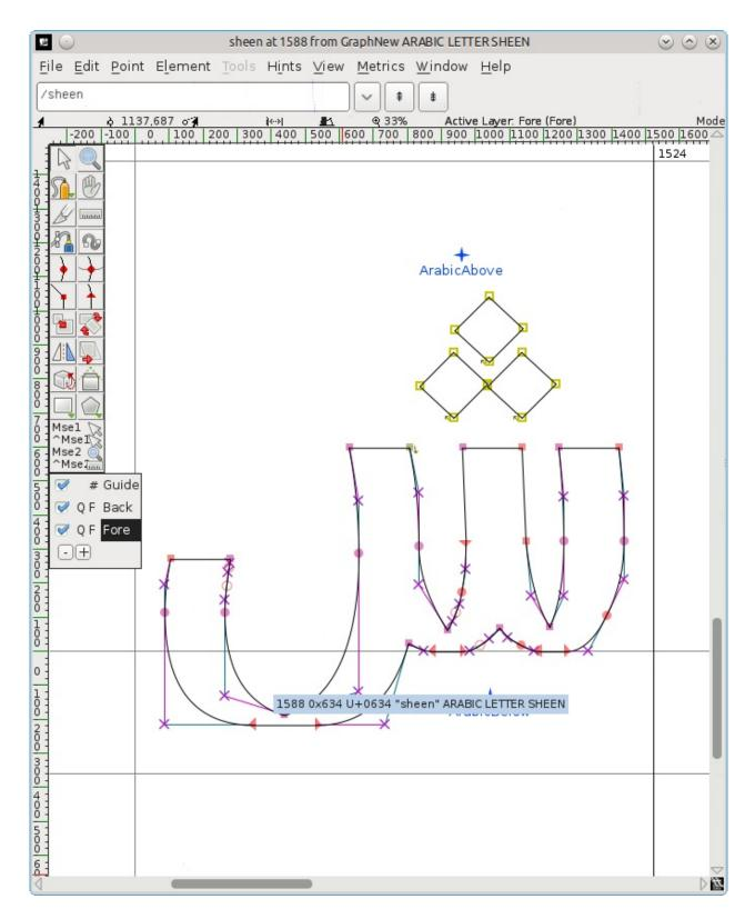
Go back to the font chart and double-click on the *peh* cell – this will load *peh* into another tab in the glyph design panel, alongside the *sheen* tab.
