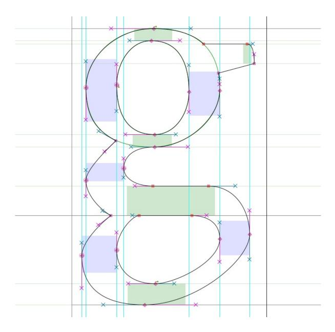
**Note:** As you can see, when setting breaks with a *Coin*, the direction of each handle should be tangent to the curve where it arrives.
