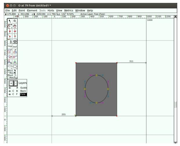
3. Go to the Element menu and choose *Correct Direction*. You will see that the two shapes merged, and that you essentially punched a hole in the center of the rectangle.
