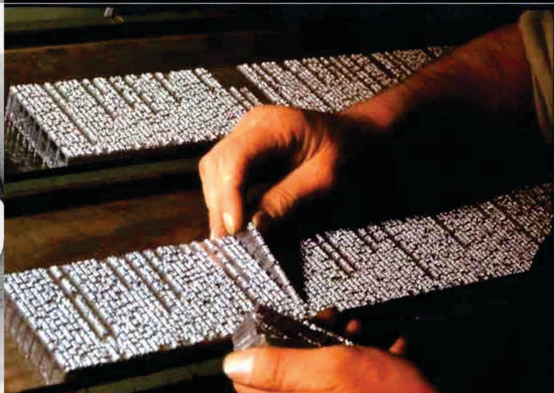
FIG. 11-1. Simplicity of handling has established the Linotype slug as the modern unit of composition.
